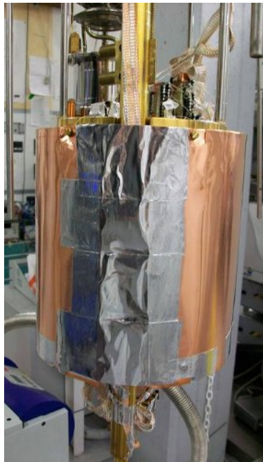
Figure 6.20: The copper shield screwed to the mixing chamber plate.
