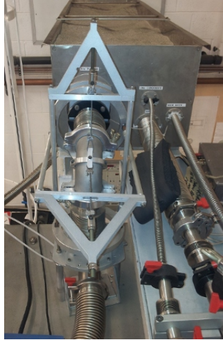
Figure 5.6: Mechanical assembly for vibration isolation (double gimbals) of the ^3\text{He} pumping line.
