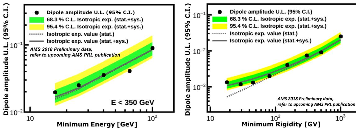
Figure 1: Upper limits on the dipole amplitudes of positrons (*left*) and protons (*right*). The points show the AMS measurement, the solid(dashed) lines correspond to the isotropic expectation with(without) systematic uncertainties, and the bands display the 68.3% and 95.4% C.L. regions.
