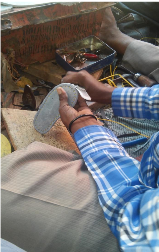
7 A shoe-maker cutting the sandal's sole out of a camel leather layer.
