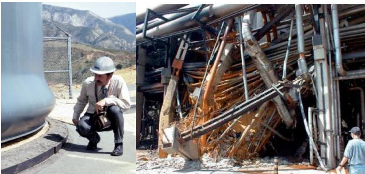
**Fig 1: Left, elephant-foot-buckling of a tank due to the del 17 January 1994 earthquake in Northridge, California; right, pipelines failure during 7 August 1999 earthquake in Tupras, Turkey [source: <http://www.enea.it/it/comunicare-la-ricerca/events/tohoku-1lug11/20110701ENEAServa.pdf>]**
