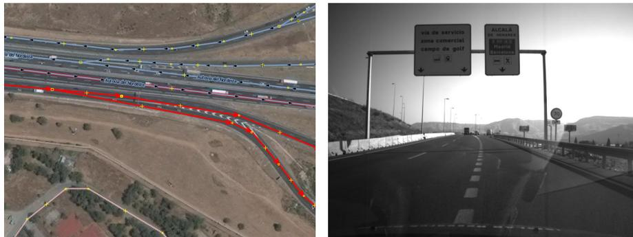
Figure 3.17: The figure depicts a common highway scenario with two parallel roads. In these cases, a simple map matching algorithm is not able to discriminate the correct vehicle position.
