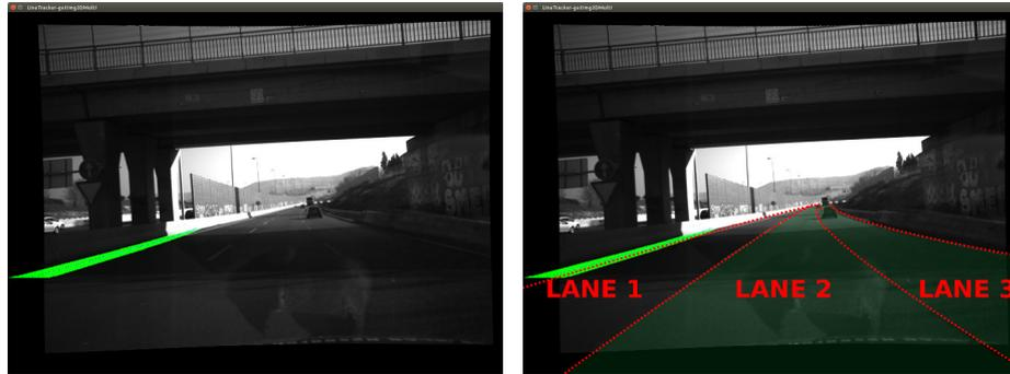
Figure 3.20: In this situation, only one out of four lines are detected. In Figure 3.20b the highlighted lanes correspond to the higher probability of the vehicle ego-lane, evaluated by leveraging the relative distance with respect to the only detected line.
