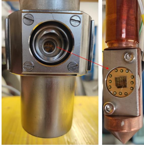
Figure 3.3: Leybold flow cryostat for electrical characterization of the devices at low temperature. An optical window allows to illuminate the device under investigation. On the right: a bonded DNPU.
