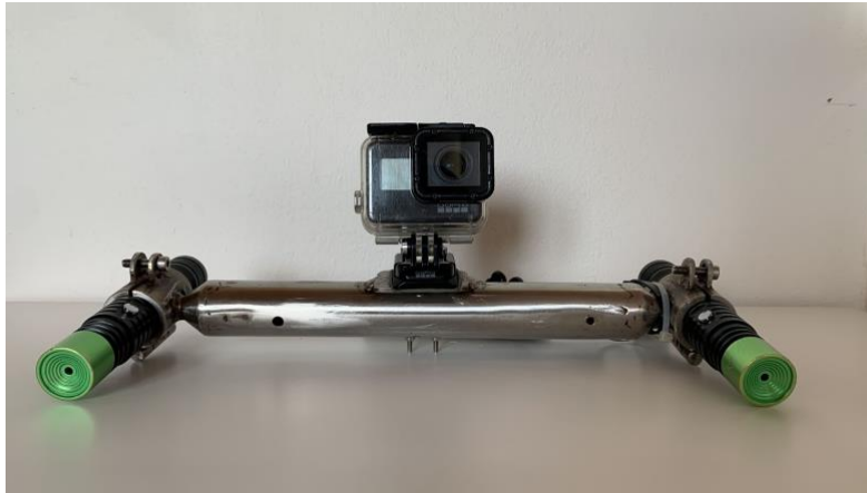
2581 Figure S1. Laser photogrammetry device used by divers collecting biometric data
