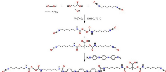
Fig. 13 Schematic synthetic pathway of DCPU. Adapted from ref. 93.
