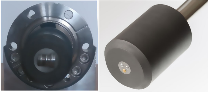
Fig. 2 Front view of the Cherenkov probe head: with the disk-like diamonds (left) and with the rod-like diamonds (right)
