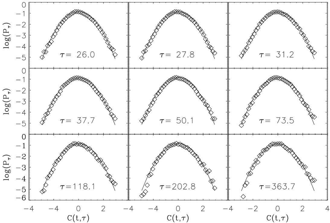
Fig.4 PDFs at different time scales (in the range 30-400 time steps) for SOC model.
