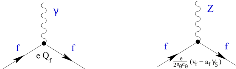
Figure 1.3: Electroweak neutral currents expected by the Standard Model. The weak neutral coupling is usually expressed in terms of vectorial and axial coefficients v_f = I_3^f(1 - 4|Q_f|\sin^2 \theta_W) , a_f = I_3^f
