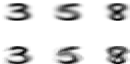
Figure 4.19: The original image of the data of the digits 3, 5 and 8 to be recognized is presented at the top while the means of the posterior produced by MCWM is presented at the bottom.
