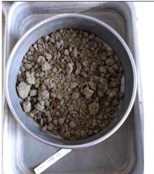
Fig. 3.4 Sieve with soil sample (Crotti bachelor thesis).
