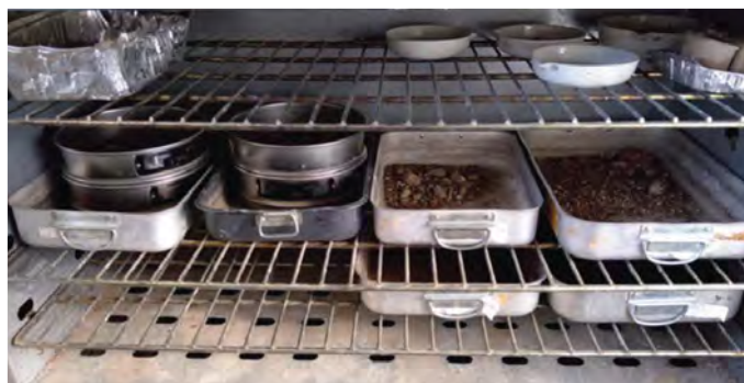
Fig. 3.7 Drying of samples inside a stove (Crotti bachelor thesis).
