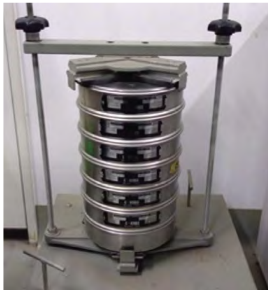
Fig. 3.5 Vibrating screen with stacked sieves (Crotti bachelor thesis).
