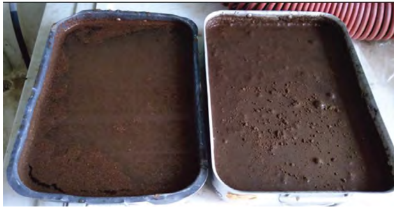
Fig. 3.6 Sedimentation of the soil inside aluminium trays (Crotti bachelor thesis).
