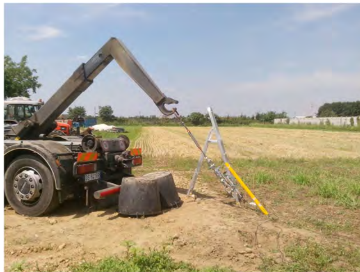
Fig. 7.13 Phase 6 - Check resistance of the anchor.
