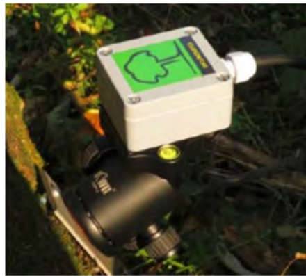
Fig. 2.3 Adopted instrumental equipment for pulling test: small scale inclinometer (Fakopp, 2020).
