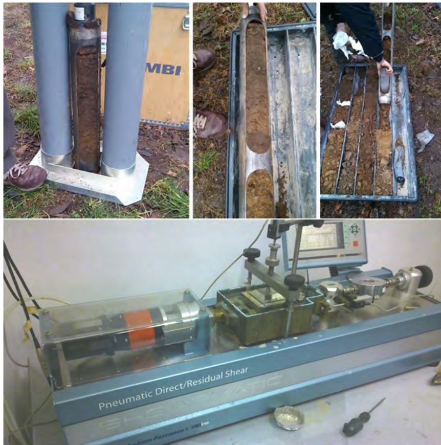
Fig. 7.6 Phase 3 - Definition of strength and deformability parameters - laboratory tests
