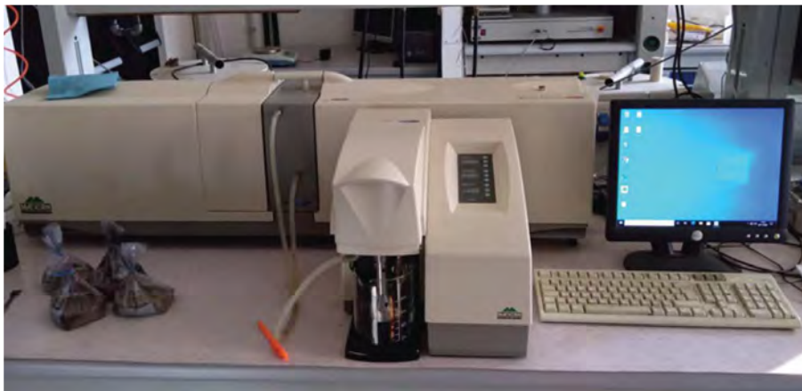
Fig. 3.8 Laser granulometer “Mastersizer 2000” by “Malvern Instruments” (Crotti bachelor thesis).
