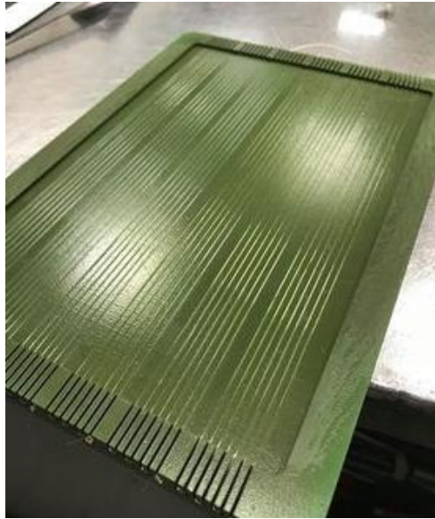
Figure 10 Monofilaments in the mold
