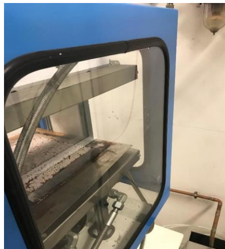
Figure 16 Pellets of Pa12 in the press
