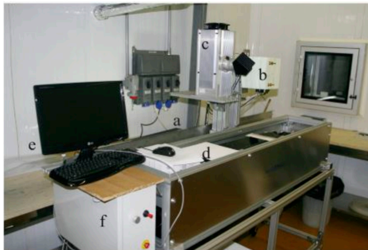
Figure 2. Picture of the system used to acquire the hyperspectral imagery. The system consists of: (a) samples holder and motor driver; (b) HeadWall VNIR camera thermostated by heaters; (c) stable halogen lamp; (d) calibrated Lambertian Spectralon panel; (e) PC connected to the spectrometer by a dedicated interface.
