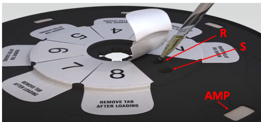
Figure 13. Liaison MDX (A) and DAD (B). DAD is characterized by a “R” and “S” wells, in which the reaction mix and sample are loaded respectively. After valve openings, the centrifugation force allows both sample and mix to reach amplification chamber “AMP”, where RT Q-LAMP can start.
