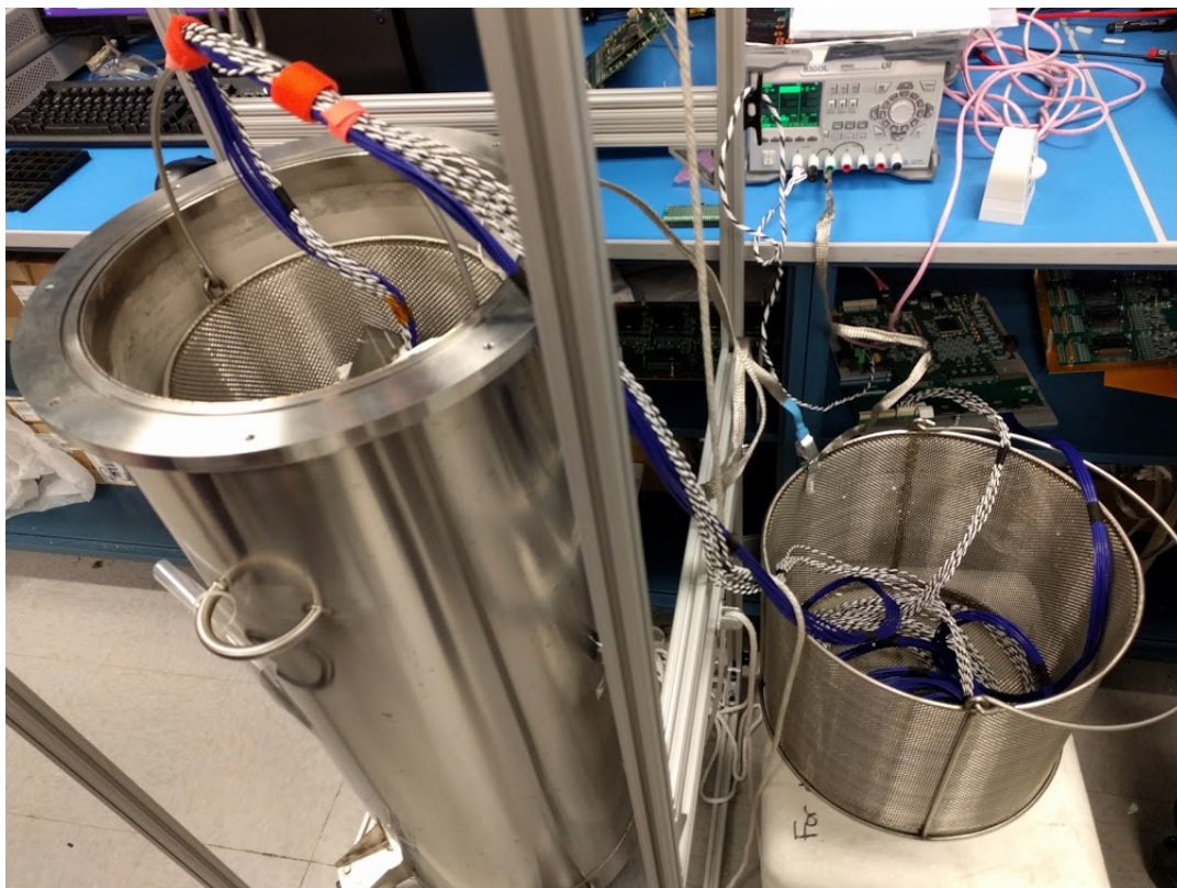
Figure 16: The FEMB production test stand, showing LN2 dewar, mesh bucket containing the CE Box inside the dewar, cold cables and WIB board. The code cables are held inside another wire mesh bucket outside the dewar during to minimize electronic noise pickup.
