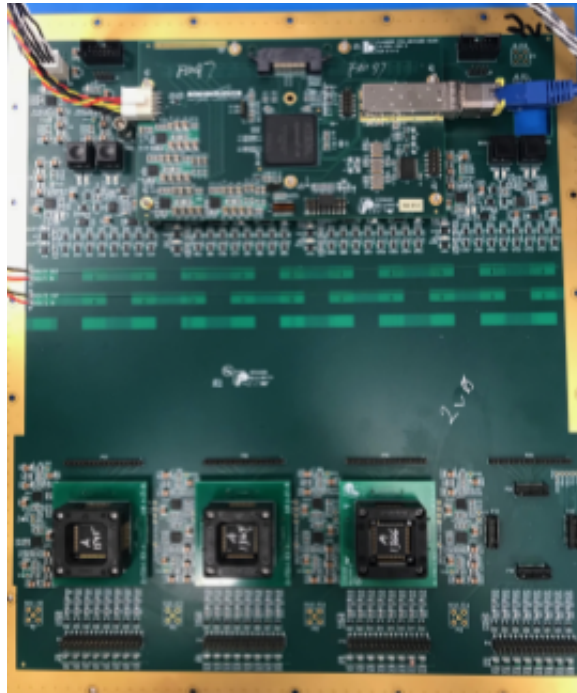
Figure 11: Quad-socket FE ASIC test board for cryogenic testing with three of four ASIC sockets installed. The additional distance between the ASICs and digital electronics improved ADC reliability by preventing them from becoming too cold to operate correctly during a cryogenic test.
