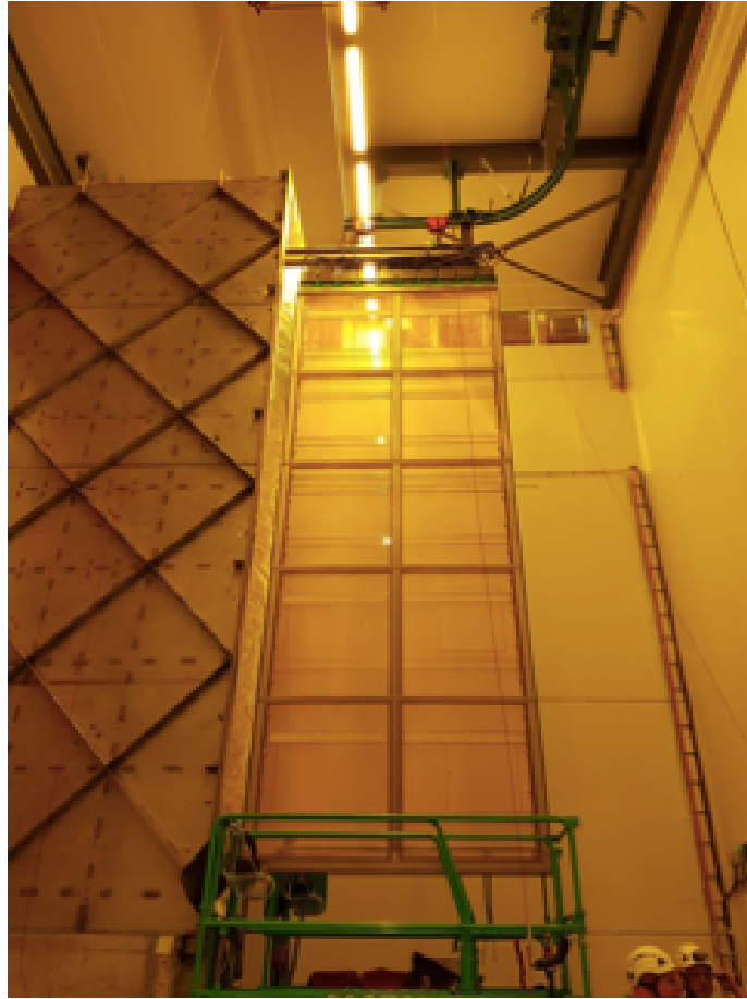
Figure 20: Picture of the Cold Box facility for APA integration test. In the picture, the APA-assembly (APA+CE system+PD system) is ready to be inserted into the cold box. On top of the APA you can also see 10 out of 20 installed CE boxes.
