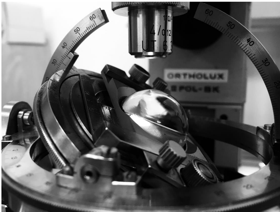
Figure 3.2. Universal stage used for quartz c -axis measurements.
