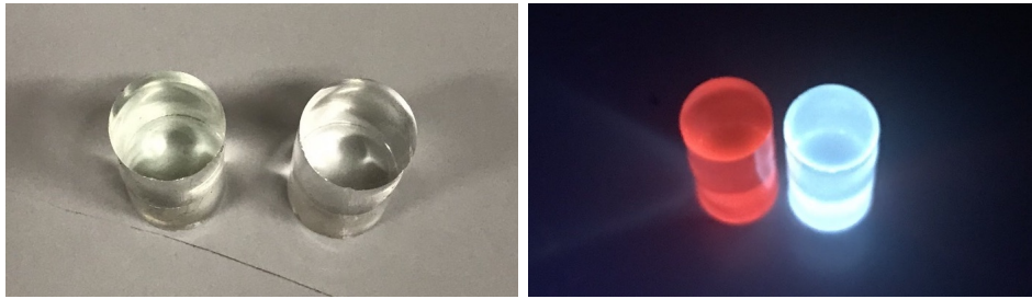
FIGURE 3.1: Pictures of Pr- and Ce-doped sol-gel silica preforms under visible light (left) and under UV light (right). Pr-doped silica (on the left of each picture) shows a greenish, although transparent, color because of the presence of Pr as dopant ion. If excited with UV light it emits in the red, due to the f - f transitions: its d - f transition occurs in a region of the UV spectrum not visible to the eye. Ce-doped silica has a blueish emission because of its 5d - 4f transition peaking at around 500 nm.
