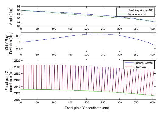
**Figure 2.4:** Chief rays are generally not normal to the local surface. The upper figure shows the absolute angle of the chief ray and local surface normal, while the middle figure shows the difference between the two. The bottom figure shows schematically direction of the ray deviation.
