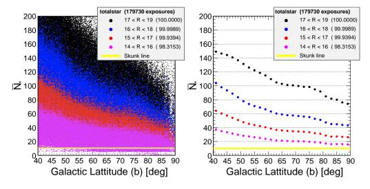
**Figure 3.22:** Total number of stars seen in six DESI GFA sensors using random pointings and the NOMAD catalog.
