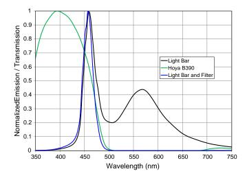
**Figure 5.19:** Spectral energy distribution of the Linear Chip On Board LED (*black*), transmission of the Hoya B390 filter (*green*), and output spectrum (*blue*).
