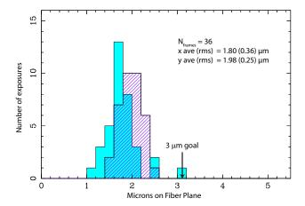
**Figure 3.30:** Distribution of the rms deviations of the FVC reconstructed fiber positions relative to their OGP measured positions. Blue is x distribution; red hash is y distribution.
