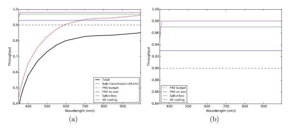
**Figure 4.2:** The predicted fiber throughput from 360 nm to 980 nm for 49.5 m of FBP fiber is shown in panel (a) and panel (b) shows the contributions that can be controlled. FRD, splice connection, and AR losses have been presumed constant with wavelength.
