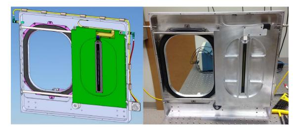
Figure 5.20: Left: Model for the Exposure Shutter shown in the open position and without one cover in place. This model shows the PneumaSeal inflateable seal around the aperture (black) and the fiber illuminator LED mounted in the middle of the shutter door (green). Right: First fabricated unit.
