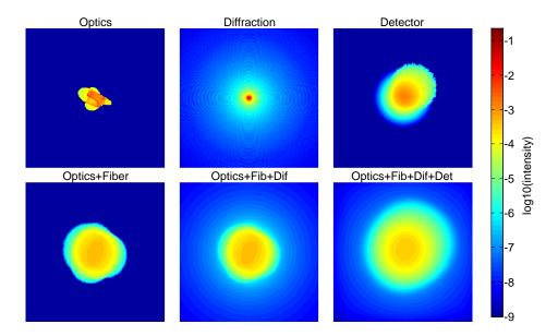
Figure 7.8: Simulated spectrograph PSF spots including various effects. Top row left to right: infinitesimally small fiber for optics only, diffraction only, detector only. Bottom row left to right:  $107 \mu m$  fiber for optics only, optics and diffraction, and optics and diffraction and detector. Each spot covers  $15 \times 15$  CCD pixels. Note that these are on a log color scale.
