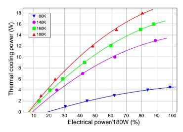
Figure 5.28: Saclay measurements of the LPT9310 thermal response for various cold-tip temperatures in a test cryostat.
