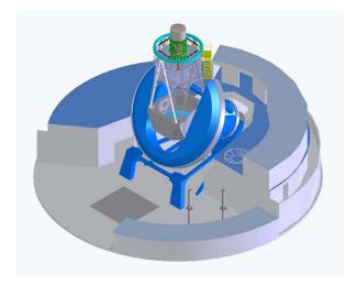
Figure 8.13: DESI top end assembly installed on telescope.
