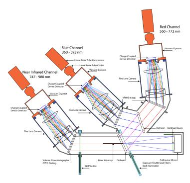
Figure 5.18: Schematic of the mechanisms of the spectrograph.
