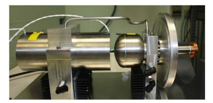
Figure 5.27: Thales 4W LPT9310 in DESI test stand.
