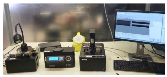
(a) splicing station showing fiber cleaver, buffer stripper, and splicer
