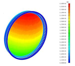
Figure 2.11: FEA model showing tilt of C4 lens and cell at a 60° Zenith angle.
