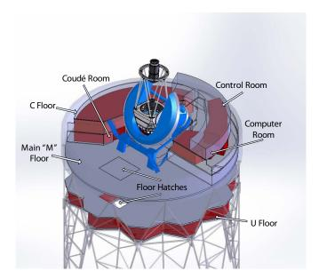
**Figure 8.2:** Iso view of the Mayall telescope at zenith pointing, showing the general layout of the major supporting facilities referred to throughout the text. The old FTS lab is on the same floor level as the Coudé room, below and behind the Computer Room from this viewing angle.
