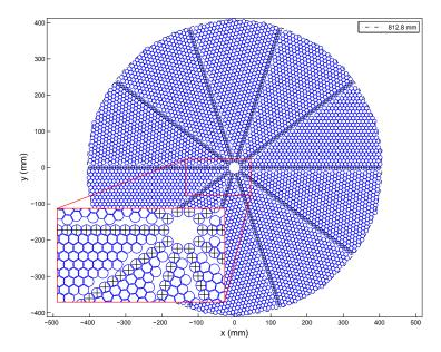
**Figure 3.5:** Typical output of fiber positioner patterning algorithm. Closeup view near center of the field is inset. "+" signs indicate locations where additional special constraints have been applied.
