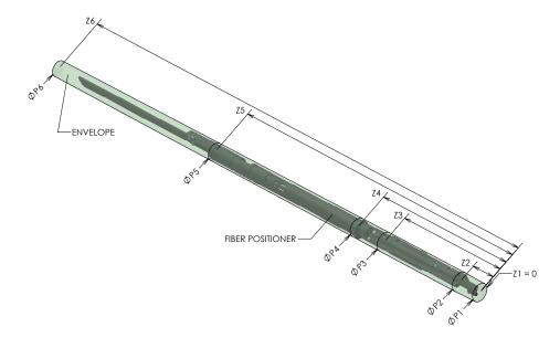
**Figure 3.4:** Mechanical envelope of fiber positioner, defined by several cones. Diameters  $p_k$  include dynamic and static tolerance stackups taken at axial positions  $z_k$ . The fiber tip is at  $z_1$ .
