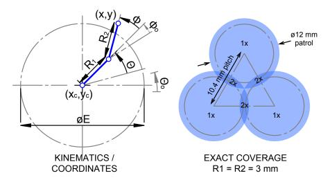
**Figure 3.11:** Left: Eccentric axis (" $\theta$ - $\phi$ ") kinematics and coordinate systems. Whenever R2 is retracted within the dashed circle E, the positioner is guaranteed free rotation about  $\theta$  without obstruction from its neighbors. Right: Patrol coverage regions for neighboring positioners. Regions labeled "1x" indicate coverage by a single positioner and "2x" by two positioners.
