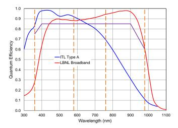
**Figure 5.35:** Quantum efficiency for DESI: ITL STA5140A and 250  $\mu$ m thick LBNL CCDs. Data are lab measurements. The purple line is the CCD specification. The vertical orange dashed lines are the locations of the band transitions for the three spectrograph channels.
