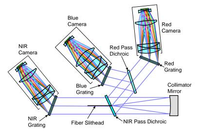
**Figure 5.1:** The spectrograph schematic.
