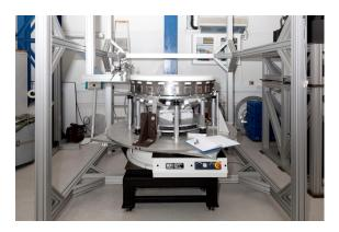
Figure 2.20: DECam C1 lens alignment setup.
