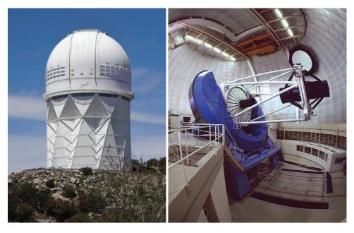
**Figure 1.1:** On the left is the Mayall 4m telescope dome structure. On the right is the telescope. The black cylinder is the MOSAIC corrector that will be replaced as part of the DESI project to instrument a 3 degree diameter field of view.
