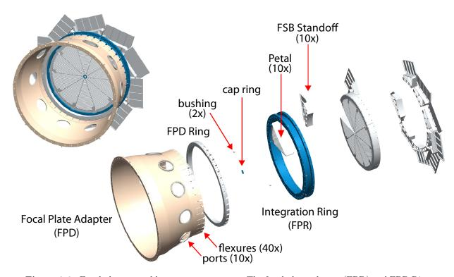
Figure 3.2: Focal plate assembly support structures. The focal plate adapter (FPD) and FPD Ring are permanently connected to one another. They form the FPD assembly, which is what connects the corrector barrel to the focal plate integration ring (FPR). Flexuring between FPD and FPD ring accommodates CTE mismatch between focal plate and barrel structure. The FPR supports the 10 petals. Each petal supports a standoff plate, where its fiber spool box (FSB) and control electronics are mounted.
