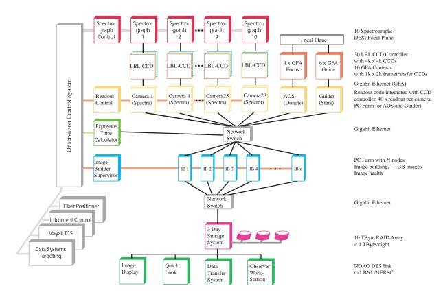
Figure 6.4: Block diagram of the DESI data acquisition system.
