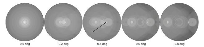
**Figure 2.6:** Images showing the complete set of two-bounce focal ghosts present at the Echo 22 focal surface for five field points. The arrow points toward the brightest focal ghost feature, a reflection between the two ADC lenses. In a 14,000 degree survey, reflections of the 1575 brightest stars along this ghost path contaminates 0.036% of the sky area with irradiance greater than 1% of NIR sky background.
