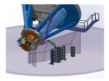
**Figure 8.16:** Fiber routing through wall of Coudé room to spectrographs. Note that spectrographs will be arranged in five short stacks and not the two tall stacks shown here.
