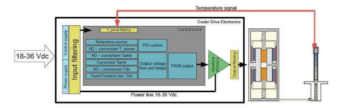
Figure 5.29: LPT9310 cooler drive electronics block diagram.
