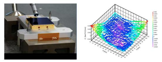
Figure 5.37: Left: CMM touch probe measurements of the package flatness for a completed mechanical grade device. Right: Deviations from the best fit plane on the mechanical grade device.
