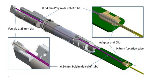
Figure 4.7: Positioner Fiber Assembly.
