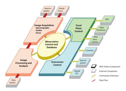
**Figure 6.1:** Schematic view of the DESI readout and control system. The observer console and other user interfaces are not shown.
