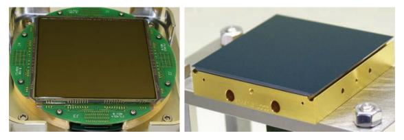
**Figure 5.34:** CCDs are  $4k\times4k$  with 15  $\mu m$  pixels. Left: ITL package for STA 4150A CCD. Right: LBNL  $4k\times4k$  CCD package.
