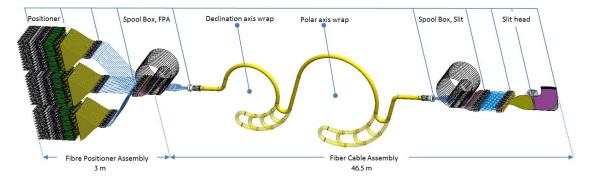
Figure 4.1: The fiber system schematic.
