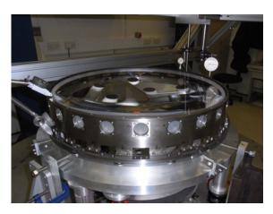
Figure 2.21: DECam C4 Lens and cell alignment setup.
