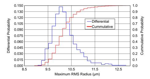
**Figure 5.12:** Statistics from the Monte Carlo simulations for the tolerancing of the red channel of the spectrograph. The blue curve is the differential probability distribution and the red is the cumulative distribution.
