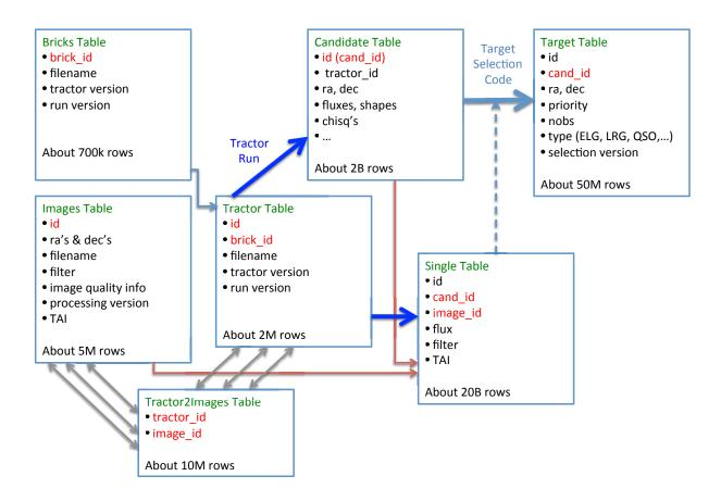
Figure 7.2: Block diagram of target selection database schema.
