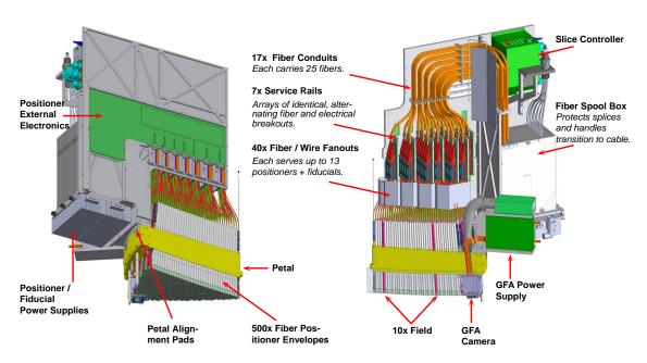
**Figure 3.7:** Illustration of completed petal assembly with fiber positioners, fiducials, GFA, and fiber spool box. This is a single unit ready for loading into the integration ring.
