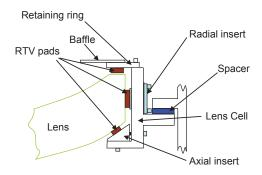
Figure 2.10: Schematic of N-BK7 lens cell design.
