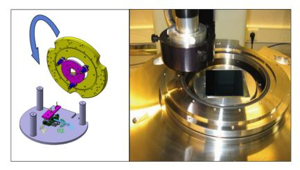
**Figure 5.33:** Left: 3 axes stage tool for precise positioning of the CCD. Right: optical machine used for CCD position measurements in the Saclay class 100 clean room.
