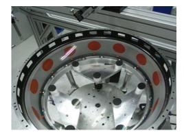
**Figure 2.8:** Mounting of the DECam optics. Shown at left is a pad and insert, and at right the radial and axial pads attached to the lens.
