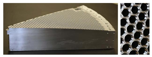
Figure 3.3: First positioner focal plane petal on left. Hole detail is shown on right.
