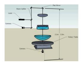
Figure 2.22: Laser alignment schematic.
