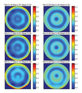
**Figure 2.3:** Geometric blur is shown as a function of zenith angle. Top figures: zenith. Middle figures: 30° zenith angle. Bottom figures: 60° zenith angle. Numbers above figures are FWHM blur in arcsec.
