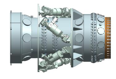
**Figure 2.13:** This picture shows the DESI corrector barrel with the DECam hexapod attached to the barrel. The hexapod configuration for the DESI barrel is very similar to the one for DECam.
