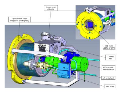
Figure 5.24: 3D model of the cryostat and view of the front side interface.
