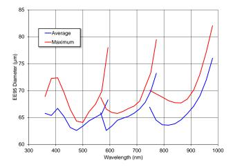
**Figure 5.15:** The maximum diameter of the 95% encircled energy versus wavelength for the simulated spectrograph. The requirement is  $< 110 \mu \text{m}$ .
