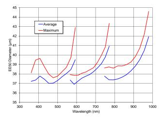
**Figure 5.14:** The average (blue) and maximum (red) diameters of the 50% encircled energy versus wavelength for the simulated spectrograph. The requirement is  $< 50\mu$ m.
