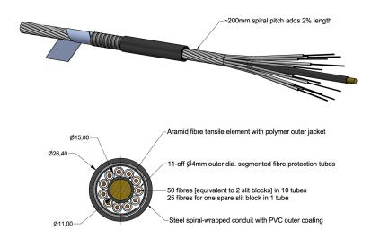
Figure 4.10: Proposed Fiber Cable cross section.
