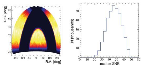
**Figure 3.23:** Left: Sky coverage for guiding SNR study. Right: Simulated median signal-to-noise for guide stars over a wide range of conditions.
