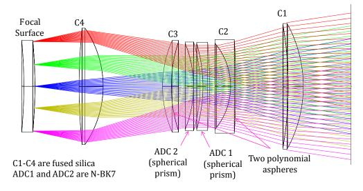
Figure 2.1: Optical layout of Echo 22.
