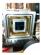
**Figure 5.38:** Left: Test Station 1 (TS1). The illumination source consists of a power regulated broad-band lamp, automated monochromator and filter wheel, shutter and integration sphere. An x-ray source is located inside the vacuum vessel. Right: Test Station 2 (TS2). TS2 with a mechanical grade 4k x 4k DESI CCD mounted inside the vacuum vessel. The optical window has been removed to show the sensor inside. The front of the image shows the confocal light source.
