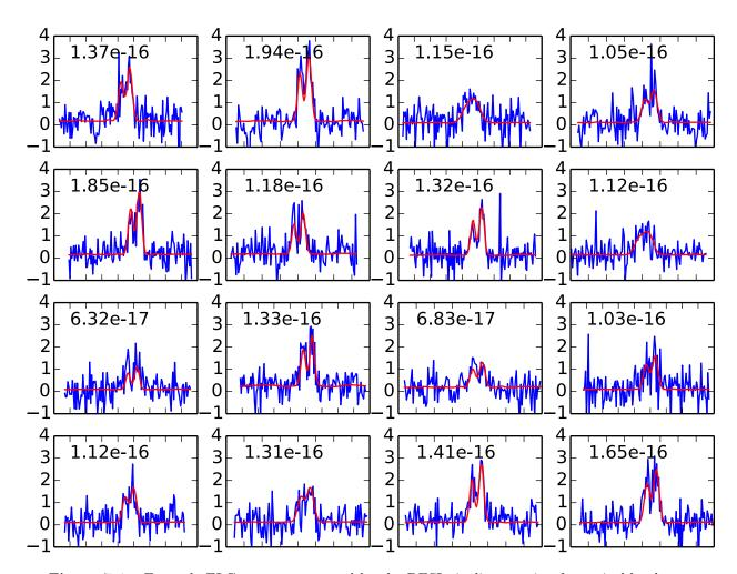
**Figure 7.4:** Example ELG spectra extracted by the DESI pipeline starting from pixel-level raw data simulations. The inset number is the [OII] flux in  $erg/s/cm^2$ . Blue shows the extracted calibrated flux  $[10^{-17} erg/s/cm^2/\text{Å}]$  vs. wavelength; red shows the input truth.
