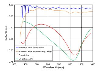
**Figure 5.2:** Reflectance of silver versus aluminum. The orange curve is for silver has reported by BOSS and used during the spectrograph design. The blue curve is a DESI measurement from the first collimator. Two types of Al are also shown as the red and green curves.
