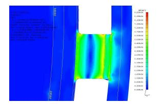
Figure 2.12: FEA model showing stresses in C2 flexure with a temperature change of  $40^{\circ}$ C.
