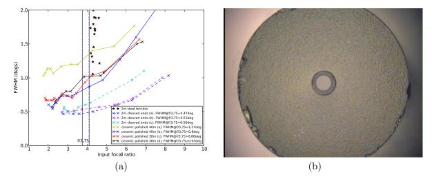
**Figure 4.8:** Collimated FRD for different methods of fiber termination. The horizontal axis shows the input focal ratio and the vertical axis shows the collimated FRD (FWHM, deg). Fibers finished with steel ferrules are shown as stars, fibers with ceramic ferrules are shown with a solid line, fibers that have been cleaved are shown with a dashed line. The vertical lines bound the f/# input range, f/3.75 to f/4.25, found at the DESI focal plane.
