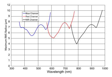
Figure 5.9: The maximum rms radius versus wavelength for the optical design is plotted. The blue, red and black curves are for the blue, red and NIR channels of the spectrograph respectively. All wavelengths meet the 10  $\mu$ m rms requirement for the optical design.
