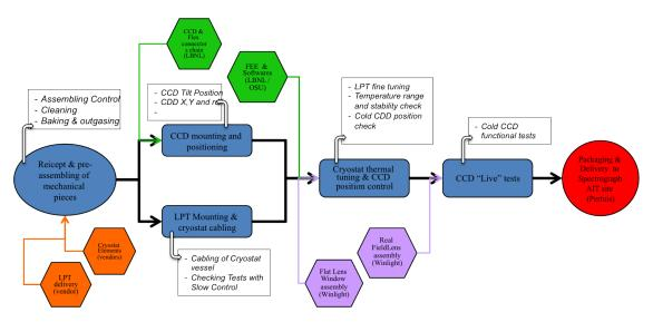
Figure 5.32: Cryostat integration Flow.
