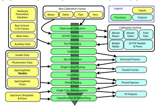
**Figure 7.3:** Schematic processing flow of the DESI DRP conceptual design. Successive steps receive data from previous steps either through intermediate data products or through direct API/function calls.
