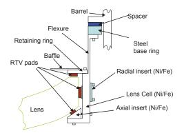
Figure 2.9: Schematic of fused silica lens cell design.
