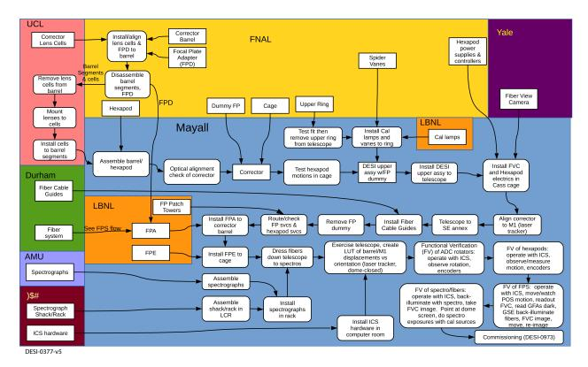
Figure 8.1: High-level DESI Integration and Test flow
