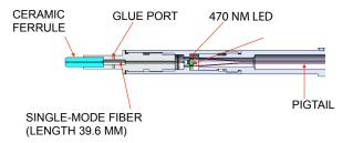
Figure 3.25: Illuminates fiducial cross section.
