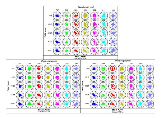
**Figure 5.8:** The ray traced spot diagram for the spectrograph. The lower left figure is for the blue channel, the lower right figure is for the red channel and the upper figure is for the NIR channel. For each figure different fiber locations are shown from top to bottom (from 0.0 to 60.5 mm) and different wavelengths are shown from left to right. The circle is the size of the projected fiber onto the detector.
