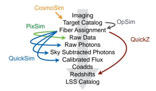
Figure 7.7: Diagram of different types of simulations under development for DESI.
