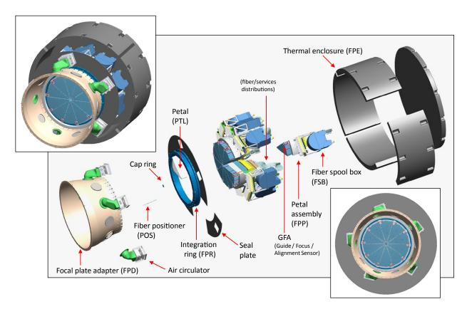
**Figure 3.1:** Illustration of the Focal Plane System. The Fiber View Camera, located at the primary mirror, is not shown.
