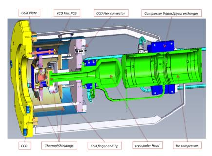
Figure 5.26: Cryostat cross sectional view.
