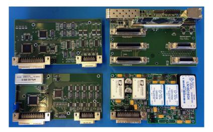
**Figure 5.39:** CCD frontend electronics module components supporting both n- and p-channel CCDs. Boards clockwise from top right are: backplane with Xilinx FPGA card, network connectors, and connector to the CCD (on the backside); controller power supplies; clock-level drivers and substrate HV voltage generator; and CCD DC bias voltages generators, preamps, and 4-channel ADC.
