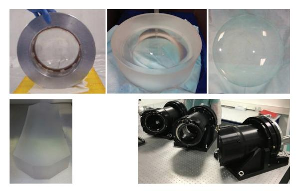
**Figure 5.11:** Photographs of several prototype spectrograph components. : The test oil cell for the blue camera. C: 200 mm diameter L2 lens for the red camera. D: 180 mm diameter L1 lens for the red camera. E: Various camera barrel components. F: The three lens barrels for the red, NIR and blue cameras.
