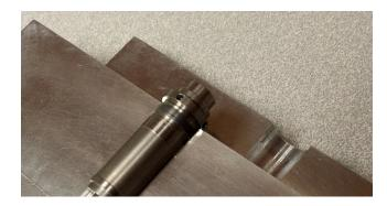
**Figure 3.6:** Left: Drill test blocks for positioner interface in 6061-T6 aluminum (rear) and 4140 alloy steel (front). Hole sizes, spacings, and tilts were machined at correct scales. Right: Section of a machining sample of the "sparkplug" style positioner retention feature. A typical precision bearing cartridge from an eccentric axis positioner is shown mated in the threads and registering below to the precision bore.
