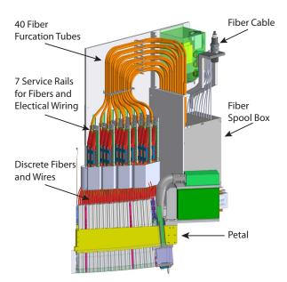
**Figure 4.9:** The focal plane is modularized via 10 petals, each holding 500 fibers. The fiber cables that contain the fibers are routed to the spool boxes in a way that allows each petal to be individually installed and removed if necessary. Fibers between the spool box and the focal plane are managed via focal plane hardware in order to ensure that the minimum bend radius requirement is not violated.
