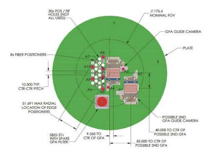
Figure 3.33: ProtoDESI focal plate layout.
