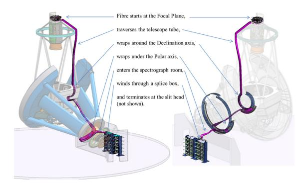
**Figure 4.11:** The routing of the Fiber Cable starts at the Focal Plane Spool Box, traverses the telescope tube and pivots, enters the spectrograph room, and terminates at the spectrograph spool box. Two routing options are shown with the one on the left preferred.
