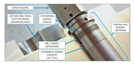
**Figure 3.12:** Positioner mechanical interface to focal plate. During insertion, the precision cylinder (g6 tolerance) of the bearing cartridge engages the precision hole (H7 tolerance) in advance of the threads. This keeps the threads well-aligned so that they engage smoothly every time.
