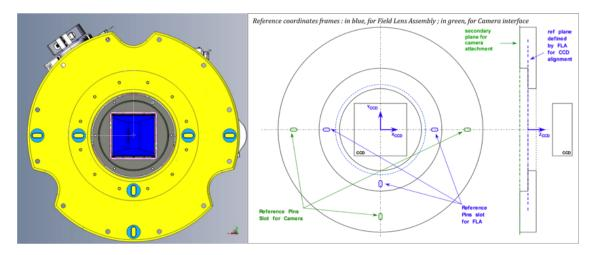
**Figure 5.25:** Reference frames system for the Cryostat Interface (blue for FLA, green for the spectrograph interface).
