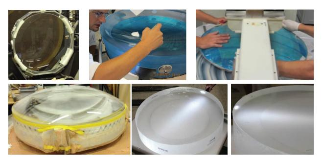
**Figure 2.7:** The six corrector lenses are show in various phases of fabrication. From top left to bottom right: C1 C1 in transmission test, C2 concave (spherical) side being checked during final figuring, C3 convex surface being polished, C4 ready for final figuring, ADC1 blank, and ADC2 being machined.
