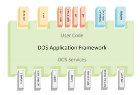
**Figure 6.6:** Schematic view of the DOS Application Framework. The Framepwork provides standardized access to DOS services such as the Architect configuration system, the DOS cloud (shared variables) and the messaging system (PML). The user provided pieces are shown on the top.
