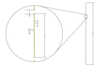
Figure 4.15: Fiber Slit geometry.
