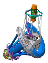
**Figure 8.15:** Fiber routing on telescope, illustrating locations and space requirements for the Dec and HA cable wraps.
