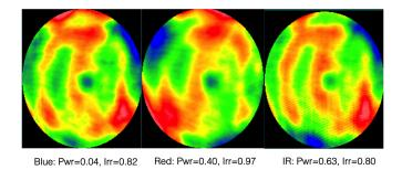
**Figure 5.5:** Measured blue, red and NIR grating wavefront in -1 order, from left to right. Power and Irregularity wavefront are indicated by Pwr and Irr, respectively.
