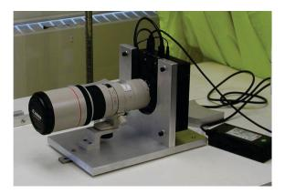
Figure 3.29: The prototype Fiber View Camera.
