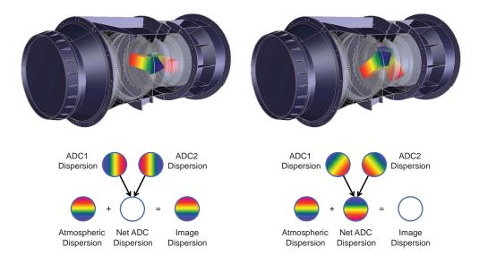
**Figure 2.2:** The atmospheric dispersion compensator consists of two oppositely oriented prisms (figures at left) which produce leftward and rightward dispersions that exactly cancel each other. Prism pairs can be rotated in opposite directions to produce a net dispersion opposite to that of the atmospheric contribution. Left and right components still cancel (figures at right), but allow a variable net dispersion that can be selected to negate atmospheric dispersion.
