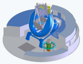
**Figure 8.12:** DESI prime focus cage installed in top ring on dome floor.
