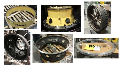
Figure 2.16: Barrel pieces as being fabricated during February 2016. Counterclockwise from the top left plot we see the Shroud, the Front section, the Middle section, the After section, the FPD and the FPD Aluminum ring.
