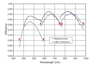
**Figure 5.6:** The vendor measured efficiency of the gratings is shown in black. The predicted efficiency is shown in blue and the requirements at the band edges are shown in red. The vendor could not measure the efficiency of the blue grating below 400 nm.
