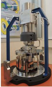
Figure 5.30: Saclay first cryostat prototype.
