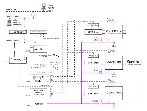
Figure 5.31: Architecture of the DESI cryostat Control System.
