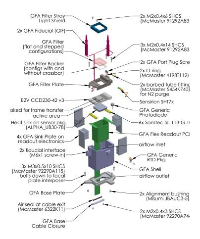
Figure 3.15: Detailed concept design for the GFA camera.
