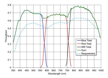
**Figure 5.16:** The estimated throughput of the spectrograph. The blue, red and black curves are for the blue, red and NIR channels respectively. The green curve is the sum of the channel throughputs and the dashed blue curve is the requirement.
