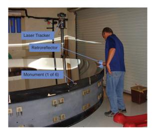
**Figure 8.3:** Laser tracker surveying of the Mayall primary mirror in July 2014. Just before realuminization, the mirror was washed and its optical surface, outer diameter, and inner hole diameter were surveyed relative to the six permanent monuments on the mirror outer diameter. This survey yielded the relation between the mirror optical axis and the fixed monuments, to help align DESI to the primary mirror.
