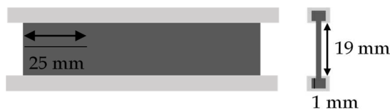
Figure 5.5. Test settings for fracture tests.
