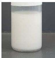
Figure 6.1. A typical sample of ZnO NPs. The suspension in hexane was stable up to one week.
