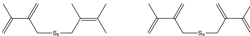
Figure 4.2. Cross-linking products composed of one or two 2,3-dimethylbutadiene units generated due to the partial oxidation of TME.
