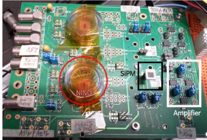
Figure 2.5: SiPM readout configuration. The positions on the PCB of the amplifiers, SiPm, and NINO timing chip (used for CTR measurements 2) are shown.
