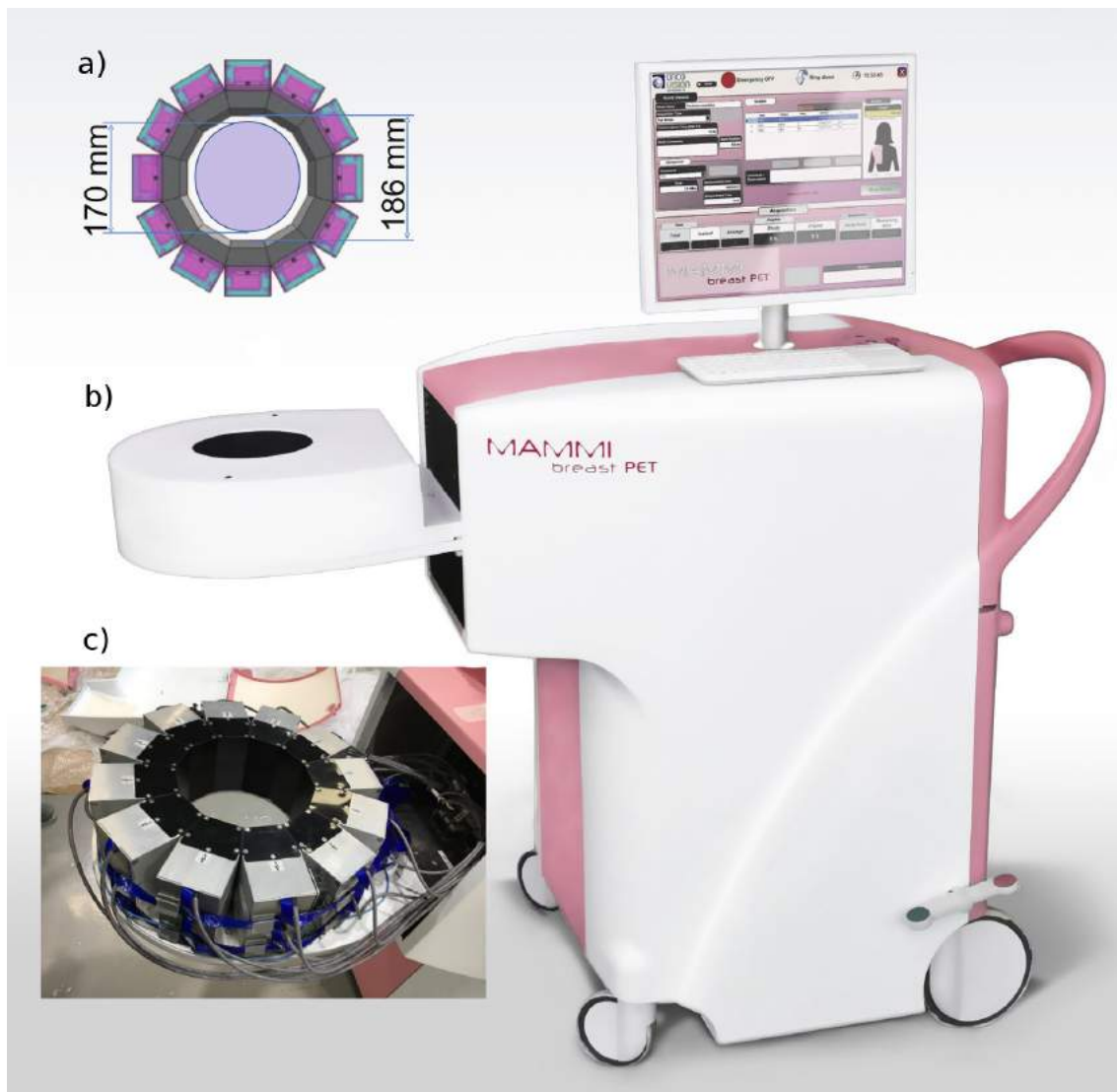
Figure 5.8: TurboPET MAMMI system. a) Detectors ring dimensions of the plastic hole diameter (170 mm) and detector ring diameter (186 mm). b) shows the machine final layout and in c) the two detector rings together.
