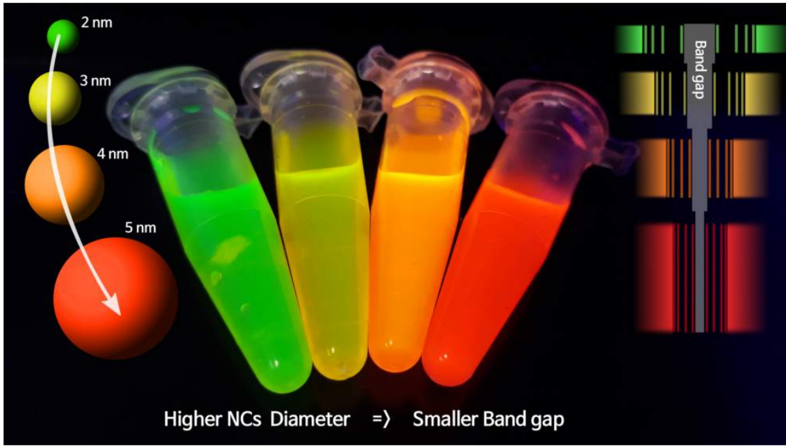
Figure 6.2: Picture of four different QDs solutions with different emission wavelengths. The QDs dimension is increasing from left to right. On the left side, a representation of the dimension trend and on the right the band gap dependency on the dimension is depicted. Smaller the NP diameter, higher the band gap and smaller will be the emitted wavelength.
