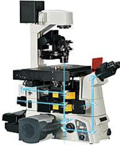
Figure 4.19.: Picture of the commercial optical microscope used for this thesis, the Nikon Eclipse Ti-E inverted microscope (Nikon Instruments, Tokyo).
