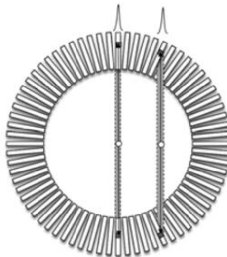
FIGURE 2.11. Effect of DOI information on spatial resolution uniformity (picture from "Positron emission tomography (PET) detectors with depth-of- interaction (DOI) capability", M. Ito et al.).
