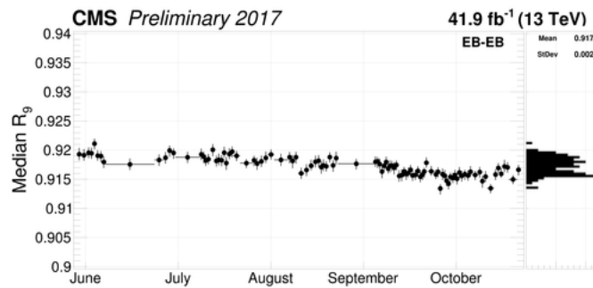
Figure 3.19: Stability of the shape of the electromagnetic deposits in the ECAL barrel for electrons from Z decays. A dedicated re-calibration using the full 2017 dataset was performed. The plot shows the stability of the variable R_9 , which is responsive to changes in pedestals and noise. Each point on the left panel is obtained by taking the median of the R_9 histogram for the respective time bin. The histogram on the right shows the spread of median R_9 . The R_9 variable is stable within 0.3% during the year.
