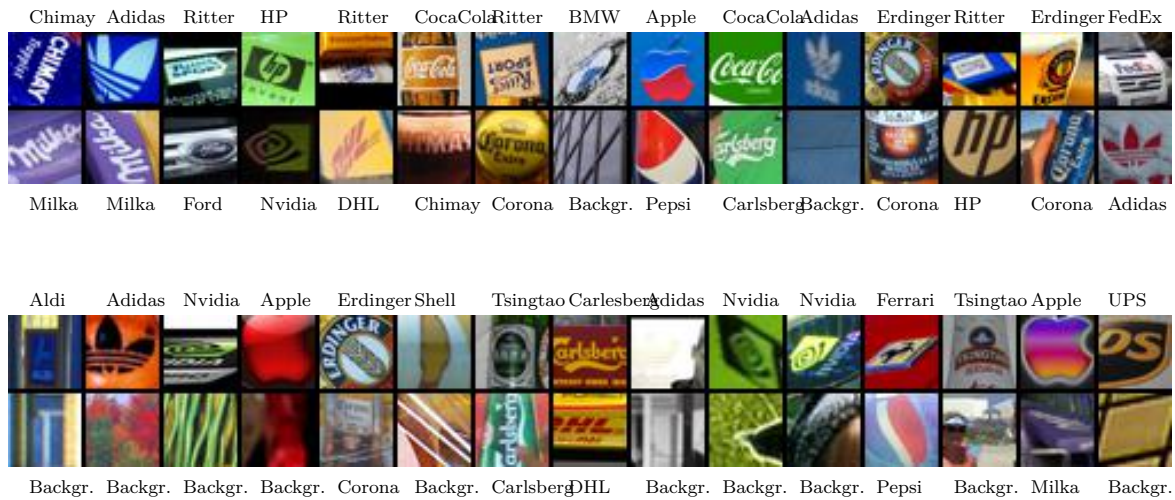
Fig. 5.15 Wrongly labeled logos ordered by confidence. Highest confidence prediction is top-left. Images resolution is 32 \times 32 pixels, i.e. the same used to feed the CNN. The first and third rows are the wrongly labeled logos, the second and the fourth rows represent the nearest example in the training set (using the last network layer activations before the softmax as feature vector).
