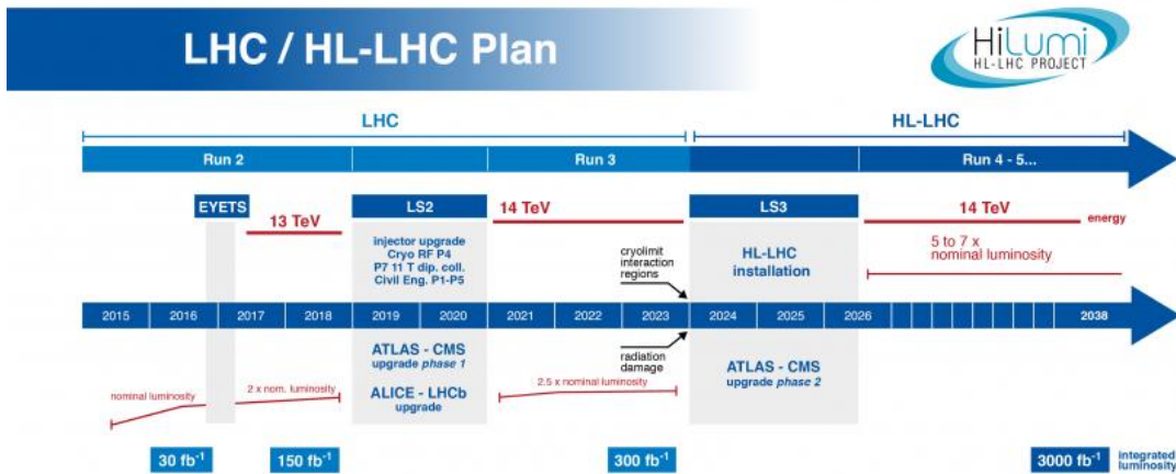
Figure 2.1: Illustration of the foreseen LHC schedule, the current phase ends with long shutdown 3 (LS3). The high luminosity phase (HL-LHC) starts after LS3 and will last for a decade. LHC standard operation includes running periods during spring, summer and fall and a technical stop for small upgrades and maintenance during winter. Larger upgrades are carried out during long shutdowns (LS), a major one will be the upgrade of the LHC and of the experiments during LS3.
