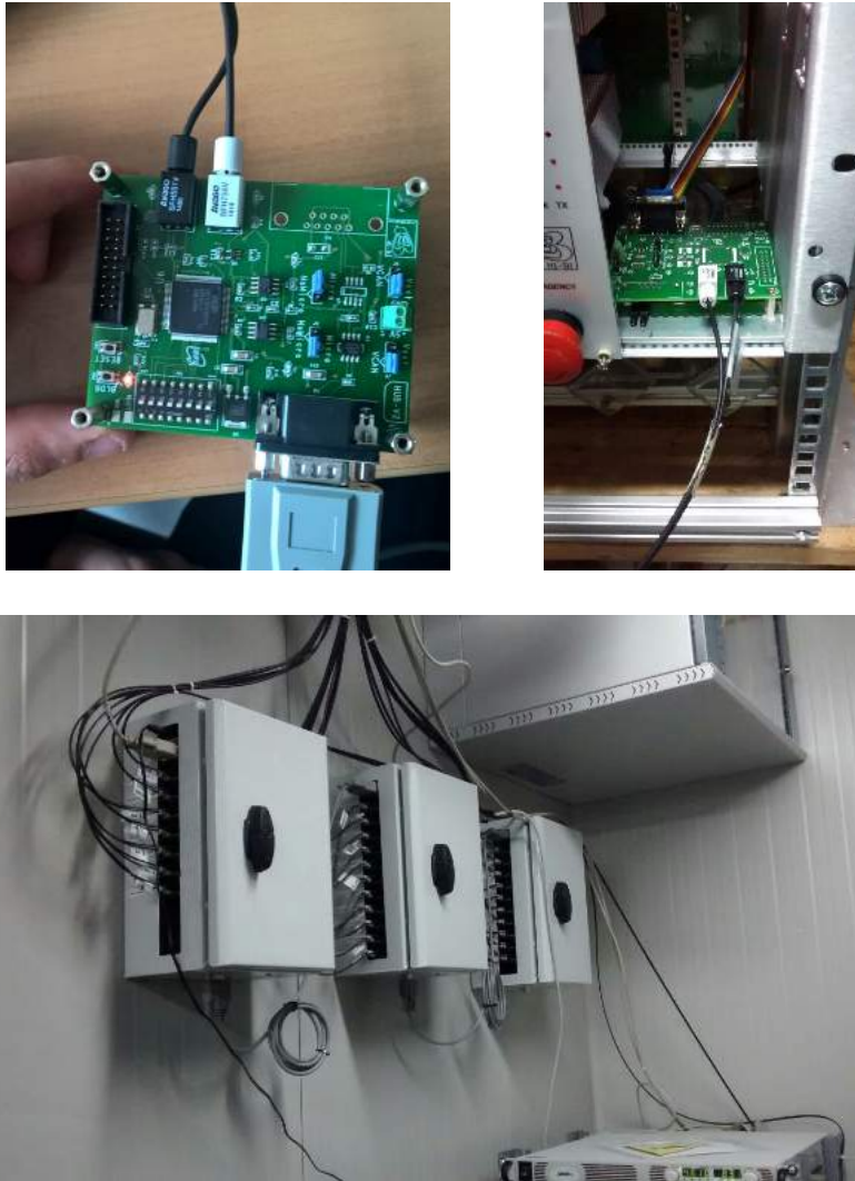
Figure 3.10: Some pictures of the HUB board. On the top-left, the HUB during the tests at the Milano Bicocca Labs. The top-right picture shows the HUB mounted as optical-to-electrical converter for a DC/DC supplier cage. On the bottom, the boxes hosting all the electrical-to-optical CAN converters which mediates the communication towards all the other devices.
