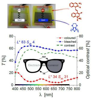
ideal candidate for application in transmissive ECDs. A proof-of-concept ECD using PB at the counterelectrode show state-of-the-art performance, combining a high lightness low saturation bleached state (L\* 83, Sab 4) with a neutral grey hue in the coloured state (L\* 34, Sab 31).
