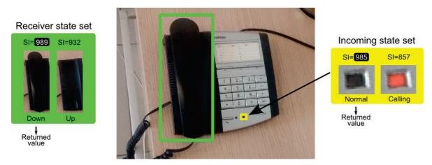
Figure 3.1: The recognition algorithm
