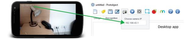
**Figure 4.2:** The smartphone displays the local IP address of the camera to be connected with Protobject desktop application.
