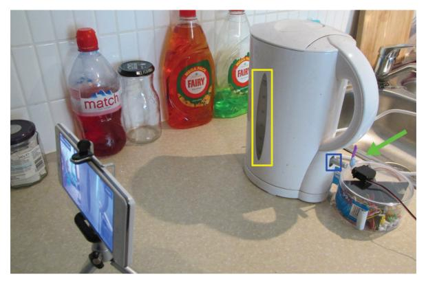
Figure 6.12: The smart boiler in which Protobject senses the liquid level and the state of the switch.
