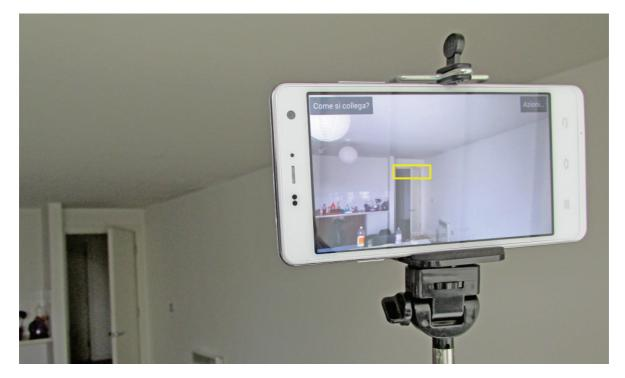
Figure 7.12: The yellow region was used for detecting the opening angle of a door.
