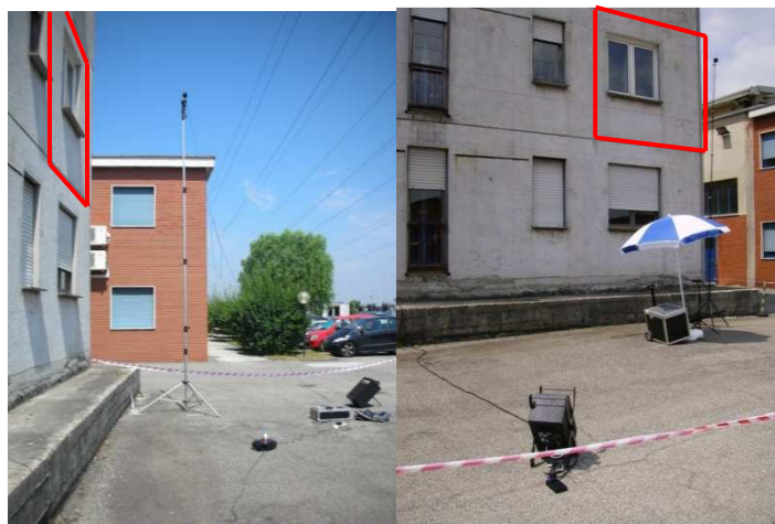
Figure 1. Different loudspeaker positions: on left side in front of the façade, on right side in a lateral position. In red the measured façade.
