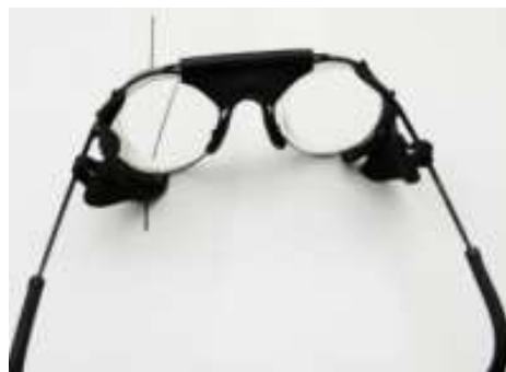
Figure 1. Goggles fitted with base-left prismatic lenses, inducing a rightward shift of the visual field.
