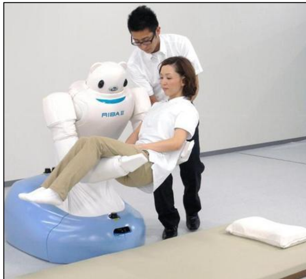
Figure 2.5: RIBA-II 1/2 , a “caregiving” robot able to lift and carry patients up to 80kg of weight.
