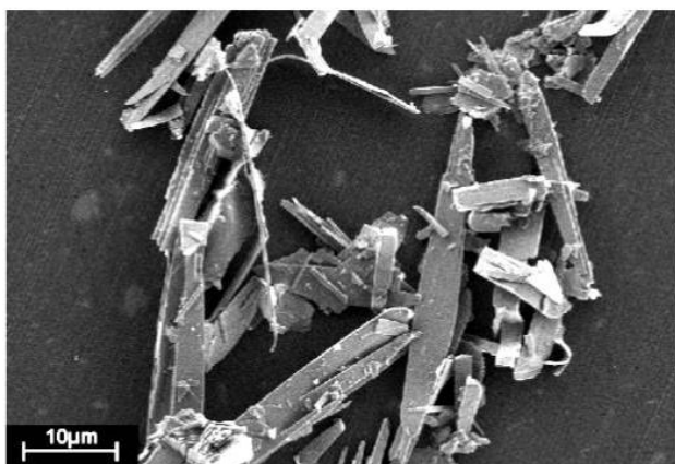
Figure B.4 | Blade-like shaped particles as a product of the solvothermal reaction of \text{LuCl}_3 .
