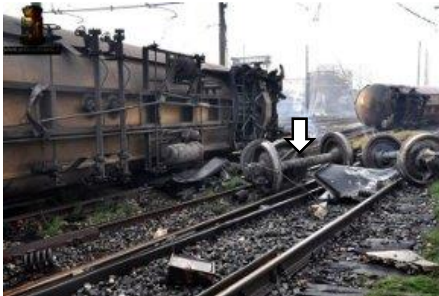
Figure 28: Viareggio accident – detached wheels-set (the white arrow indicate the axle.) 57
