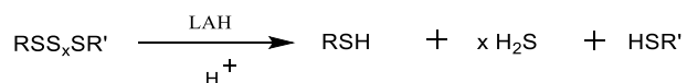
FIGURE 2.9: REACTION OF LITHIUM ALUMINUM HYDRIDE WITH DI- AND POLYSULFIDIC CROSSLINKS (ADAPTED FROM REF.[2]).
