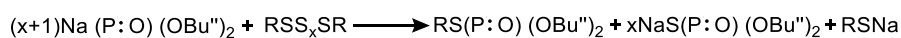
FIGURE 2.8: CLEAVAGE OF DI- AND POLYSULFIDIC CROSSLINKS BY SODIUM DIBUTYL PHOSPHITE, (ADAPTED FROM REF.[3]).
