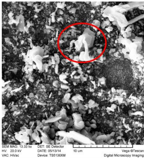
Figure 4: SEM top-view of a portion of a CZTS film. The bright agglomerate marked in red contains only Cu and S.
