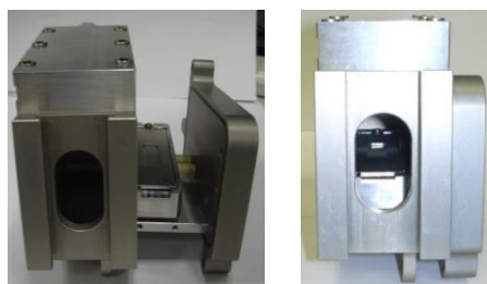
Figure 41. Target body with the aluminium plates in open and closed mode (left and right, respectively) with the window for the entrance of the proton beam during the irradiation into the cyclotron.
