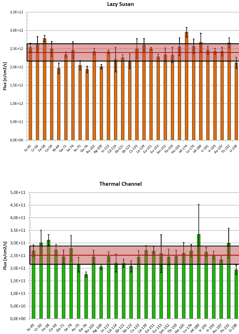
Fig. 3.4: Comparison of the neutron flux results evaluated from the data of each precursor isotope in the four irradiation facilities. The shadowed area corresponds to \pm 1\sigma range from the mean value, where \sigma is the standard deviation of the results.
