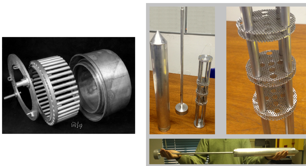
Fig. 2.8: The Lazy Susan rotary specimen rack (left) and the Thermal Channel irradiation facility with a zoom on its internal samples holder (right).
