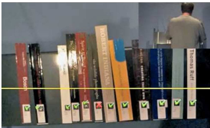
Picture 5.5 The ShelvAR App shows a book out of order, thanks to QR-codes
