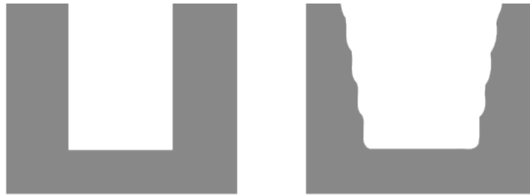
Figure A.10: Ideal directional etching ( left ); linear combination of directional and isotropic etching (with weight 5/6 and 1/6 respectively) to mimic imperfect anisotropy ( right )
