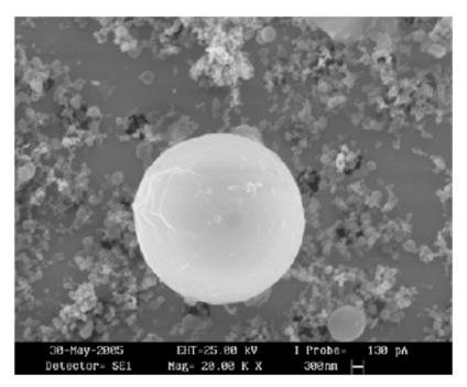
Figure 15-11: anthropogenic particle containing iron, observed in indoor sample (source ARPA Lombardia)
