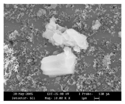
Figure 15-10: mineral particles in indoor samples (source: ARPA Lombardia)
