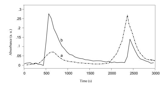
Figure 3-6: CECs obtained by TGA/FT-IR analyzing SRM1649a using a first temperature step of 350°C (curve a) and 435 °C (curve b), respectively
