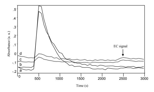
Figure 3-5: CECs obtained by TGA/FT-IR analyzing a 24-hour sample of particulate matter (on a filter). The filter was divided into two portions both heated at 425°C for 25 minutes (curves a and b). Curve c was obtained with the heating program reported in Fig. 3, on one half of the filter submitted to 24-hour Soxhlet extraction; curve d was obtained with the same heating program on the second half of the filter not extracted.
