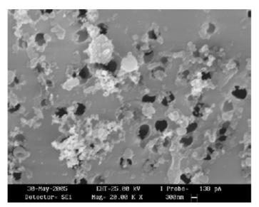
Figure 15-9: carbonaceous particles observed outdoor (source: ARPA Lombardia)
