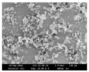
Figure 15-8: carbonaceous particles observed indoor (source ARPA Lombardia)
