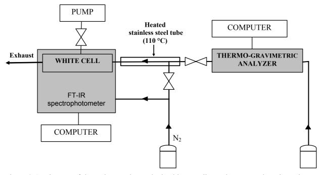
Figure 3-1: Diagram of the carbon analyzer obtained by coupling a thermo-gravimetric analyzer (TGA) with an infrared spectrophotometer (FT-IR).
