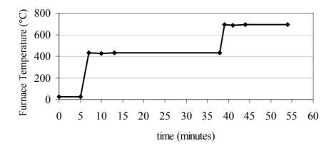
Figure 3-3: Heating program employed for the analysis of particulate matter samples by TGA/FT-IR
