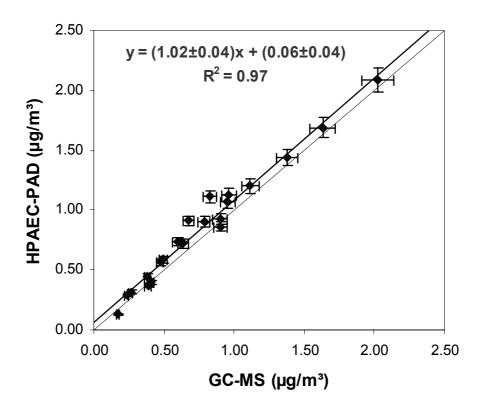
Figure 7-5: figure 5: comparison between GC-MS and HPAEC-PAD
