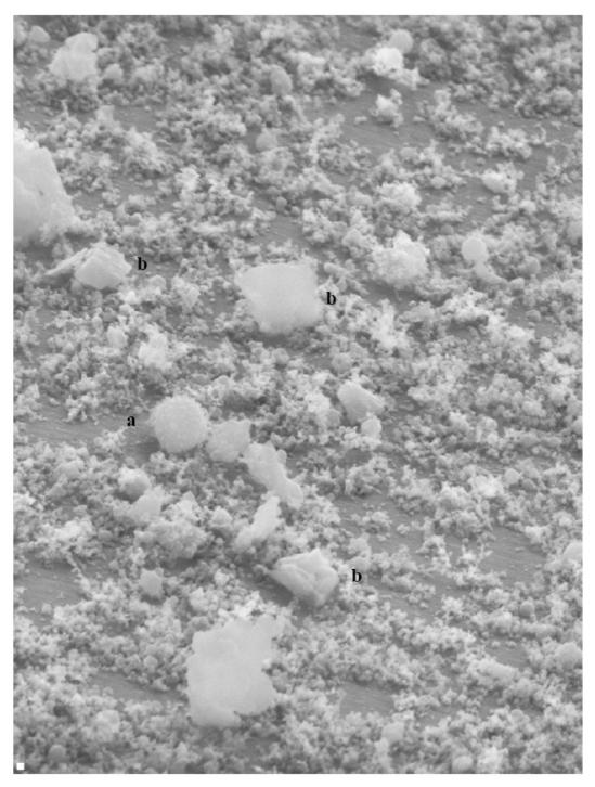
Figure 15-12: particles observed indoor sample. In the background there are much sub micronic carbonaceous particles. (a) biological particles, (b) mineral particles (source ARPA Lombardia)
