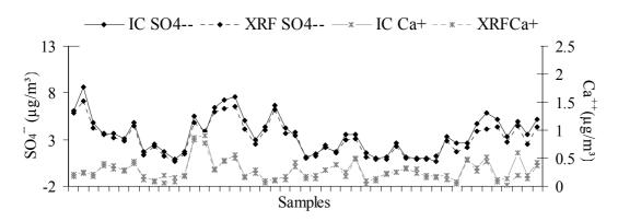
Figure 2-2 Comparison between IC and XRF data, obtained analyzing PM1 filters, for  $Ca^{2+}$  and  $SO_4^{2-}$
