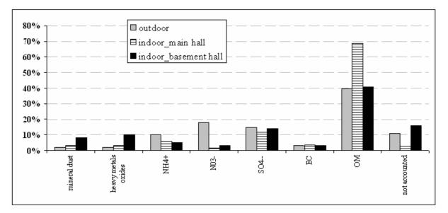
Figure 14-1: Chemical mass balance related to indoor (basement and main hall) and outdoor PM2.5 measurements.
