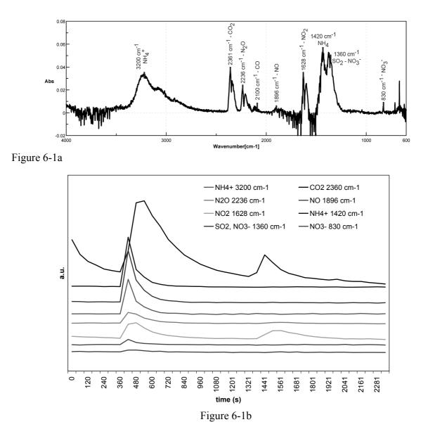
Figure 6-1 Evolution curves (b) for the different species and the corresponding IR spectrum (a)
