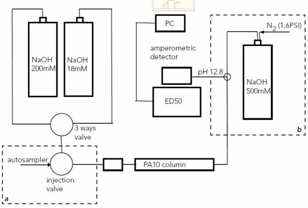
Figure 7-2: analytical set-up, upgrade of ICS 1000 - Dionex instrument
