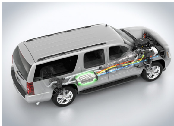
Figure 1.4: TEG prototype inserted into the exhaust system of Chevrolet Suburban. Source: General Motors
