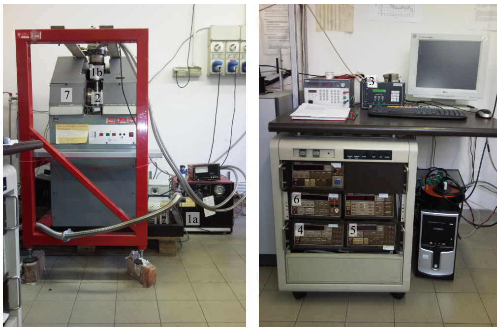
Figure 3.10: Experimental setup for resistivity and Hall measurements
