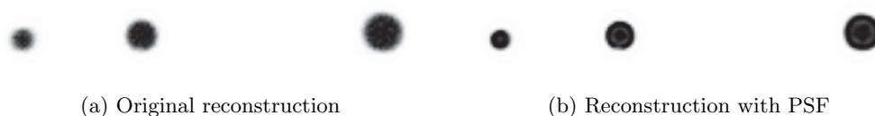
Figure 5.4: Edge effect in a reconstruction of three uniform spheres
