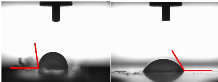
Figure 2.3: contact angles of a water drop on chlorinated polyethylene (left) and Nylon terpolyamide (right) surfaces.
