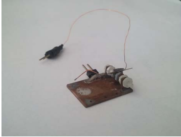
Figure 5.1: Picture of the sample holder. In this figure the tungsten tip and the electrical connections are clearly visible.
