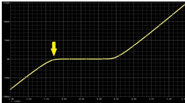
Figure 5.30: Simulated IV curve from the model reported in Fig. 5.28 with I1 generating current (illuminated).
