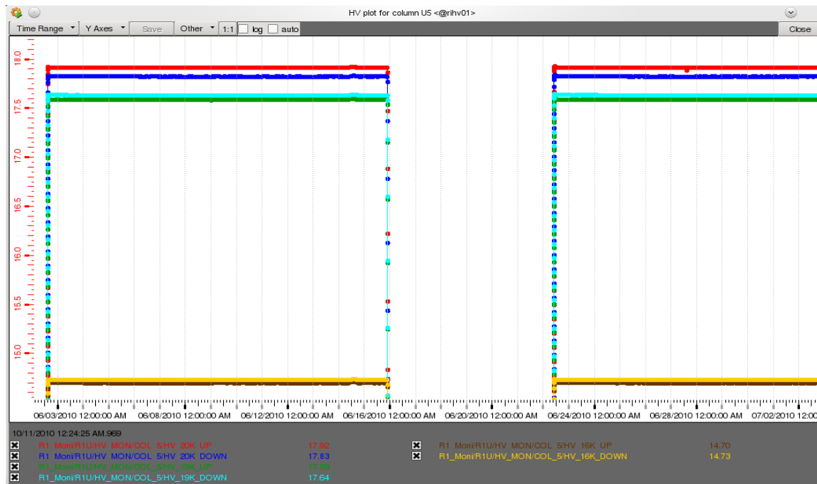
Figure 4.5: Example of a stable column: U5. Trend plot of the ELMB voltages in June 2010
