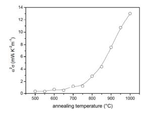
Fig. 2. Power factor of the poly layer as a function of the annealing temperature. The simultaneous growth of  $\alpha$  and  $\sigma$  lead to a maximum power factor of 13 mW K<sup>-2</sup> m<sup>-1</sup>. For the sake of comparison, Si nanowires are reported to have power factors of 3.2 mW K<sup>-2</sup> m<sup>-1</sup> [1].
