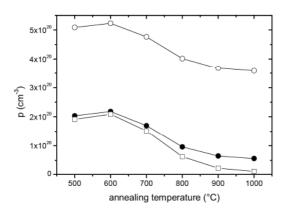
Fig. 4. Experimental evolution (filled circles) of the carrier density upon annealing (Experiment II) compared to hole density computed according to the standard Mott approximation (open circles) and accounting for the exact carrier statistics (open squares). See text for details. Lines are intended as eye's guide only.
