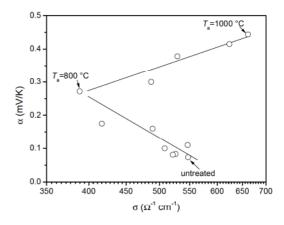
Fig. 1. Experimental variation of the Seebeck coefficient with the conductivity. For annealing temperatures in excess of 800 °C both transport coefficient concurrently grow up.
