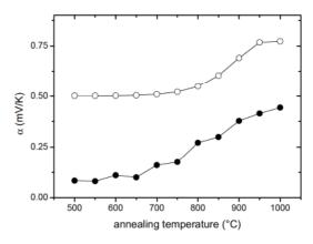
Fig. 6. Computed (open circles) and experimental (filled circles) Seebeck coefficients upon annealing (Experiment I). Lines are eye's guides.
