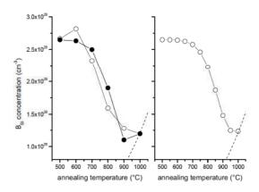
Fig. 3. Plot of *(left)* the experimental (open circles) and fitted (filled circles)  $B_{Si}$  concentration upon annealing (Experiment II); and *(right)* of the computed  $B_{Si}$  density as a function of the annealing temperature (Experiment I). The dashed line shows the solubility of  $B_{Si}$  in the single crystal [20], [17]. Full lines serve as eye's guide only.
