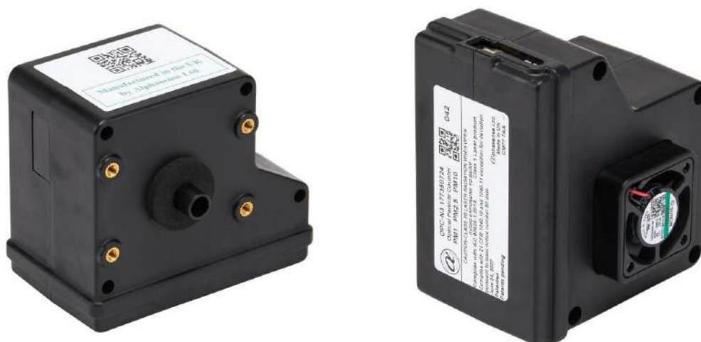
Figure 2.6. Outer case of the OPC-N3 sensor.
