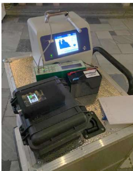
Figure 5.1. Employed sensors for the Pinacoteca di Brera and Palazzo Citterio campaigns, mounted on a moving platform to allow fast switching between sampling locations.
