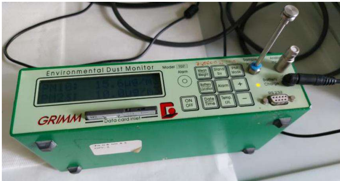
Figure 2.3. The Environmental Dust Monitor model 1.107
