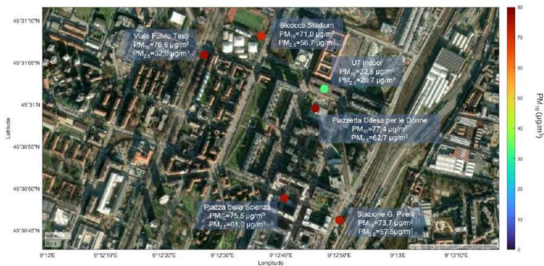
Figure 6.5. Map of the first route with average PM_{10} concentration for each sampling location obtained deploying the RESPIRO devices during the pilot campaign.
