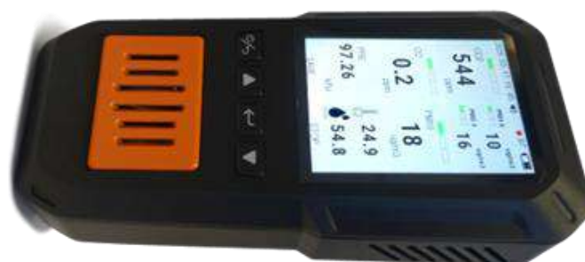
Figure 6.4. Overview of the low-cost RESPIRO device developed.
