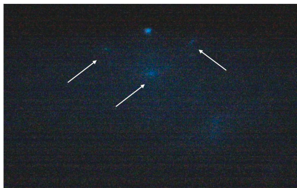
Fig. 7. The RHEED pattern during the crystallization of the sample DE10-HF. Arrows indicate short horizontal streaks originating from well-oriented vertical facets of GaAs nanocrystals.
